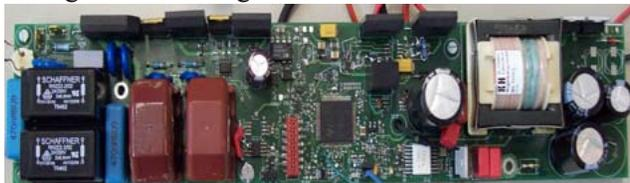
**Fig. 2: PSU system prototype**
