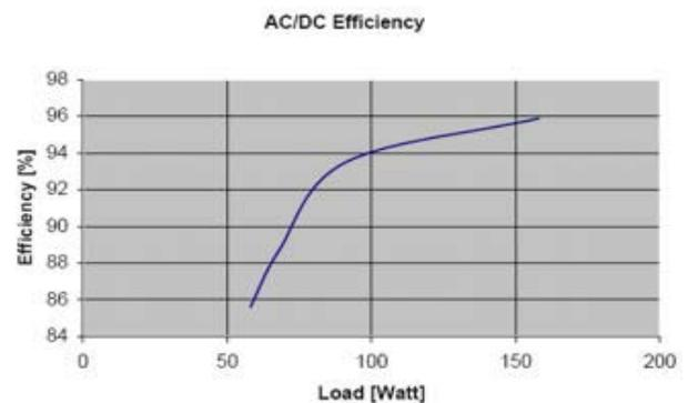
**Fig. 4: AC/DC efficiency curve**
