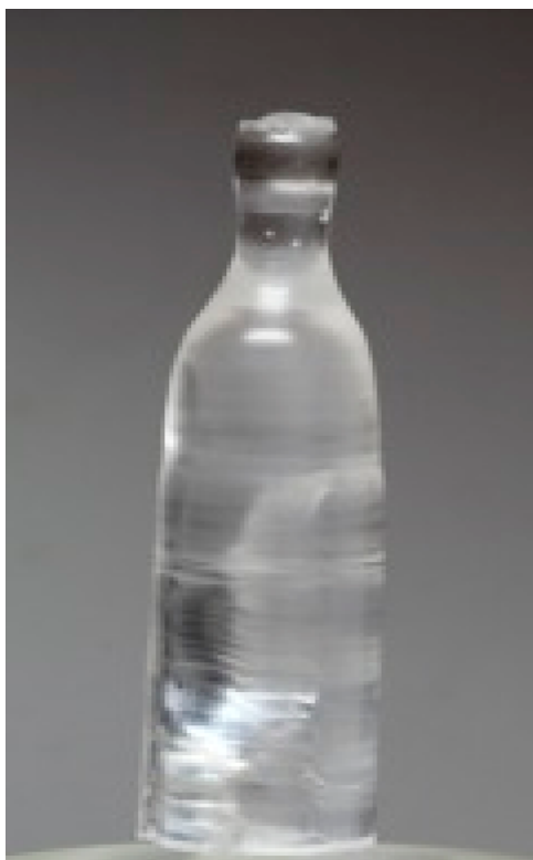
Figure 1. Czochralski grown BaCaBO 3 F ( l \approx 40 mm).
